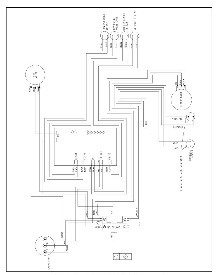
Figure 16. Typical Factory Wiring (Copeland Compressor)
